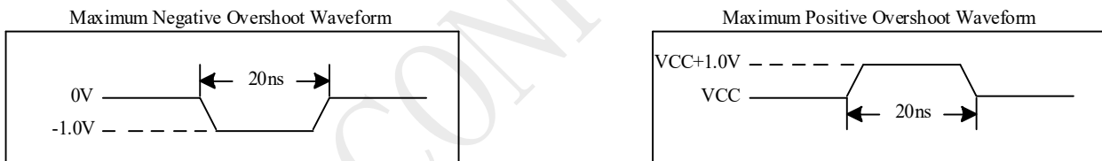
Figure 5-3 Maximum Overshoot Waveform
